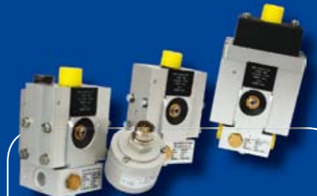
The product family SWKP MV 20 comprises dump valves with low response times for various applications. They are available with a nominal diameter of 1/2" or 1" and with pressure gauge as an option.
